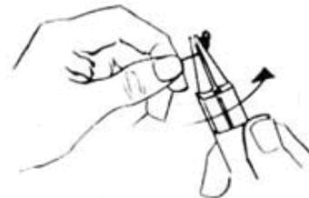
10) Hold the wire that is to be cut toward you and cut at the place indicated. Cut just one wire.
