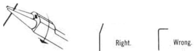
34) Grip the wire just beyond the completed bend. Bend it backwards in the exact opposite direction of the previous bend, as directed by the arrow, from left to right. Continue all the way around until you have bypassed the previous wire. This complete twist may be made easier by taking a second grip with the pliers when only half completed.
