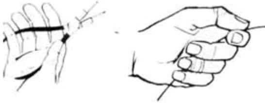
2) With pliers in the right hand, let the cutting edge face the left hand. Now grip the wire at right angle with the pliers a short distance from the tip of the pliers. NEVER ALLOW THE WIRE TO EXTEND THROUGH THE TIP OF THE PLIERS. THIS WILL MAKE OBLONG LOOPS. the more the wire is concealed within the pliers the more perfect the loop.
